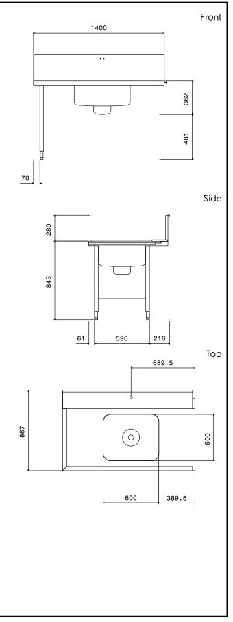
Handling System for Pot & Pans Pre-wash/Unloading Table with Deep Left Basin, 1400mm
